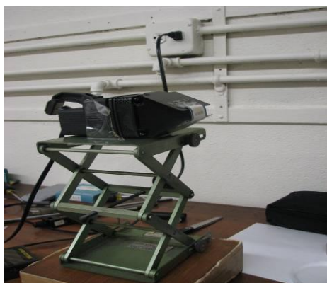
Fig. 3: Light source, attached a cardboard with a small hole to make it a point source.
