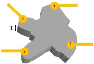
You should get two different resistances for two different sets of contacts on the edges of the sample. Definitions for the measurement:
