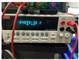
Connect to the V+/- ports on the sample. You may find it useful to press the "rate" button on the front panel to slow the rate the digits are changing- expect a good amount of electrical noise in the room, which will affect the last few digits.
