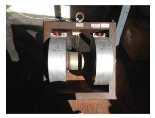
The direction of the field is labeled for current traveling in the direction of RED to BLACK. This direction is important for finding the sign of the charge carriers. This magnet is composed of two solenoids with iron cores to boost the field. Connect the current to the magnet so that it travels in one side and then the other in series.
