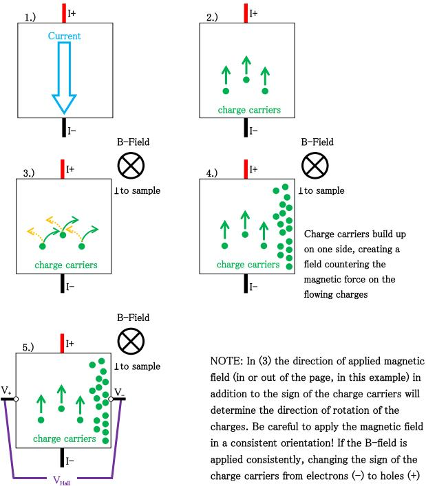
charge carriers from electrons (-) to holes (+) will reverse the sign of the hall voltagemeaning you can determine the sign of the charge carriers. The Experiment:
