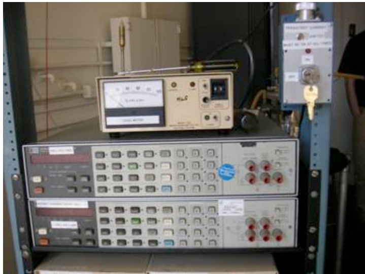
Figure 5 , Hall DVM, (middle), FIELD DVM (bottom), and PERSISTANT SWITCH BOX (r., w/ key)
