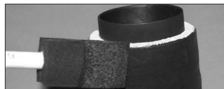
HiE-Coat™ 840-M coats exhaust pipe insulation.
