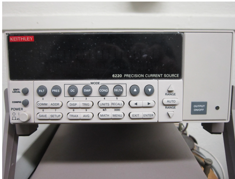
Figure 3: The control boxes for the 4-wire measurement: Top: Keithley 6220 precision current source; Bottom: Keithley 2812A nanovoltmeter; Left: Lakeshore temperature controller.
