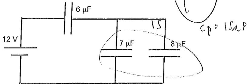
(4 points) For the circuit above, find the equivalent capacitance.
