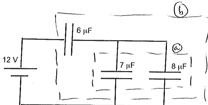
(4 points) For the circuit above, find the equivalent capacitance.
