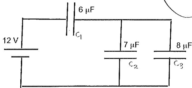
(4 points) For the circuit above, find the equivalent capacitance.
