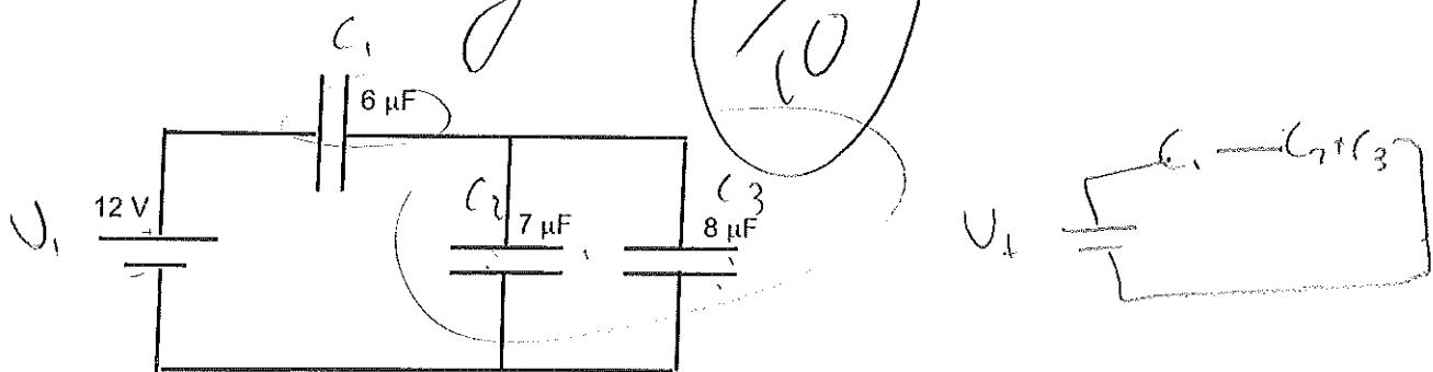
(4 points) For the circuit above, find the equivalent capacitance.
