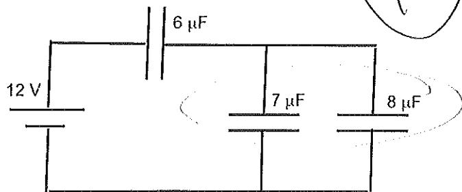
(4 points) For the circuit above, find the equivalent capacitance.
