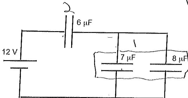
(4 points) For the circuit above, find the equivalent capacitance.
