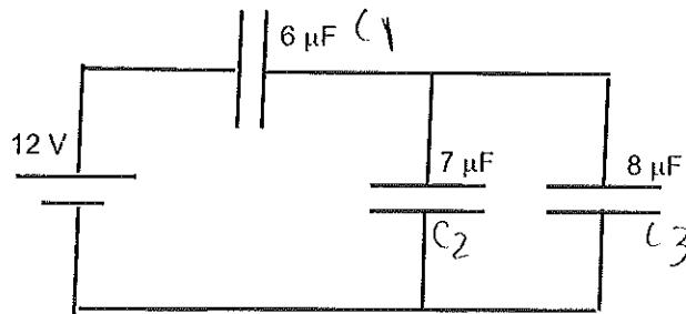
(4 points) For the circuit above, find the equivalent capacitance.
