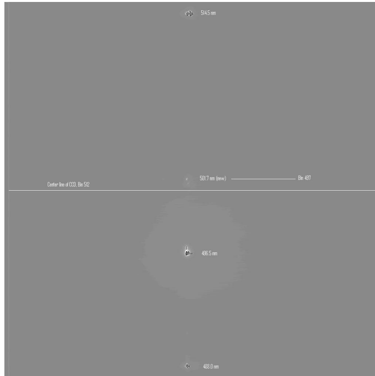
Figure 2: Second multiline calibration image. The beam is less filtered, so more lines are present. The lines from the first figure have saturated and leaked into adjoining pixels because of the longer exposure time.
