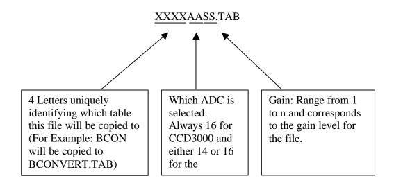
When loading the TAB files, the software should always load the information from the 8 default files listed above. If a change in the gain level or ADC is required, the TAB files for that particular ADC and gain level combination should be copied into the corresponding default files.
