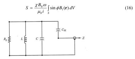
Figure 5 Series capacitive matching circuit
