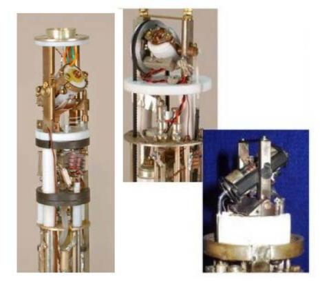
Figure 7 Three NMR Solids probes
