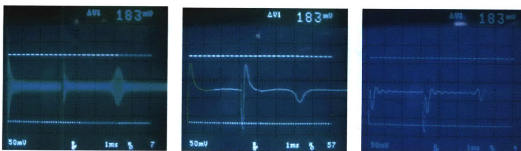
(a) Amplified NMR signal. The envelope of the FIDs and echo are clear. (b) Amplified NMR signal mixed with a sinusoid at Larmor frequency, then low-pass filtered. (c) NMR signal mixed with a sinusoid that is slightly off the Larmor frequency and filtered.
