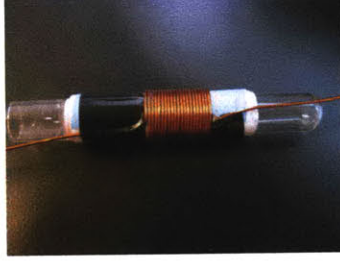
Figure 4-3: Photo of a coil being made.
