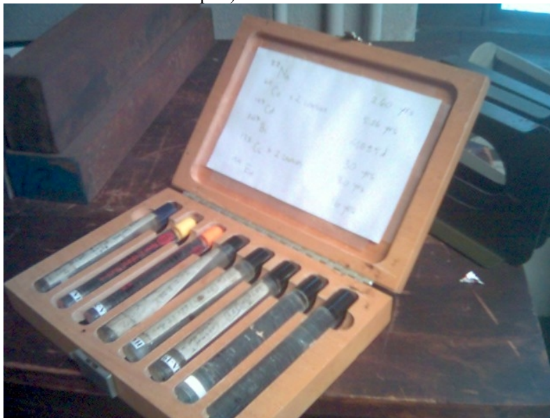
Figure 3: Sample container. The actual samples are in the black/colored piece at the ends; the remainder is a clear plastic handle by which to handle the sample.
