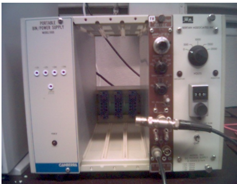
Figure 2: The power supply unit (L), signal amplifier (C) and high-voltage supply (R).
