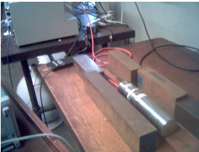
Figure 1: NaI scintillation counter, surrounded by radiation shielding blocks. The small black box behind the photodetector is the multi-channel analyzer (MCA) which interfaces with the computer. In the background are the high-voltage power supply (see Figure 2) and the computer.
