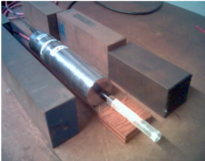
Figure 4: Correct sample alignment
