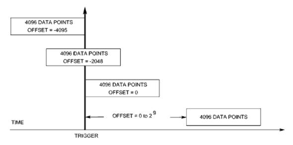
To offset the beginning of the acquisition buffer relative to the acquisition trigger:
