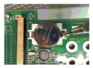
5. Install the new battery. Make sure that the positive side (+) is facing up. Place the battery *under* the small spring clips closest to the ribbon cable connector, then push down on the opposite end of the battery to seat the battery (see red arrow below). The top of the small spring clips should be visible after the battery is seated (see red circle below).
