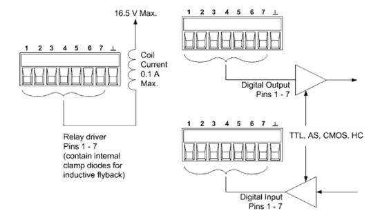
To configure the pins for digital I/O:
