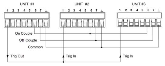
Program pin 6 as the On Couple pin; program pin 7 as the Off Couple pin. This setting is saved in non volatile memory.
