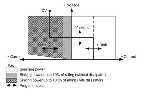
The heavy solid line illustrates the locus of possible operating points as a function of the output load. As shown by the horizontal portion of the line, the output voltage remains regulated at its programmed setting as long as the load current remains within the positive or negative current limit setting. A CV (constant voltage) status flag indicates that the output voltage is being regulated and the output current is within its limit settings.
