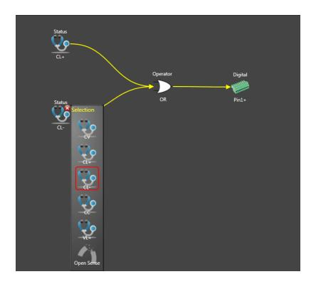
**Example 2** Create a trigger source that will trigger an output transient (step or list) whenever the output current is between 2.1 A and 2.7 A.
