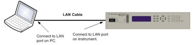
1. Connect the instrument to the site LAN or to your computer using a LAN cable. The as-shipped instrument LAN settings are configured to automatically obtain an IP address from the network using a DHCP server (DHCP is set On). The DHCP server will register the instrument's hostname with the dynamic DNS server. The hostname as well as the IP address can then be used to communicate with the instrument. If you are using a private LAN, you
