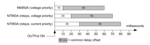
The common delay offset assures that the user-programmed turn-on delays will be synchronized to start at the completion of the common delay offset. Query the delay offset of each unit and use the slowest delay as the common delay offset.
