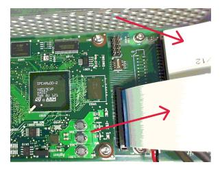
3. To access the battery, release the ribbon cables by pulling up on the locking tab.
