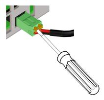
Make your connections as shown in the following figure. Connect the load to the output terminals using separate connecting wires. Keep the wire-pair as short as possible and twist or bundle it to reduce lead inductance and noise pickup. Keep load leads under 14.7 meters (50 feet) per lead because of inductance effects.
