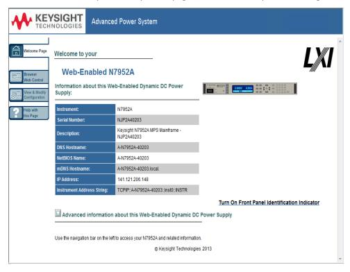
If desired, you can control access to the Web interface using password protection. As shipped, no password is set. To set a password, click on the View & Modify Configuration button. Refer to the on-line help for additional information about setting a password.
