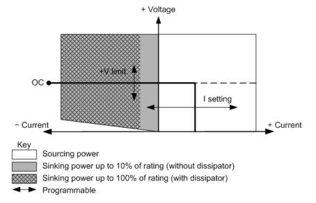
The heavy solid line illustrates the locus of possible operating points as a function of the output load. As shown by the vertical portion of the line, the output current remains regulated at its programmed setting as long as the output voltage remains within its limit setting. A CC (constant current) status flag indicates that the output current is being regulated and the output voltage is within its limit settings.
