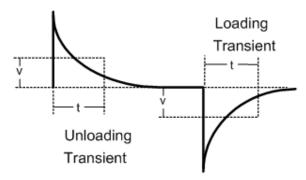
Step 7. The output voltage should return to within the specified voltage at the specified time following the 50% load change. Check both loading and unloading transients by triggering on the positive and negative slope. Record the voltage at time "t" in the performance test record form under "Transient Response".
