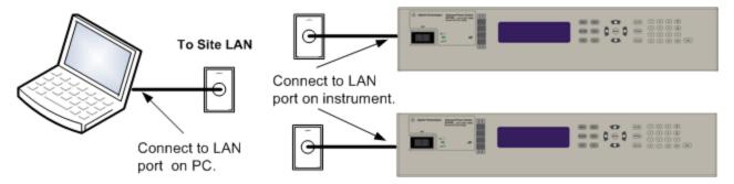
A private LAN is a network in which LAN-enabled instruments and computers are directly connected, and not connected to a site LAN. They are typically small, with no centrally-managed resources. The following figure illustrates a typical private LAN system.
