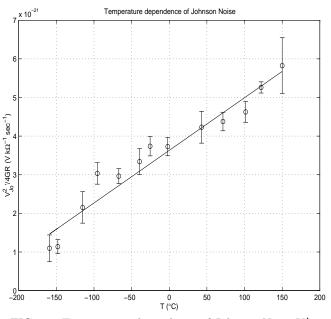
FIG. 10. Temperature dependence of Johnson Noise  $V'_{Jo}$ .
