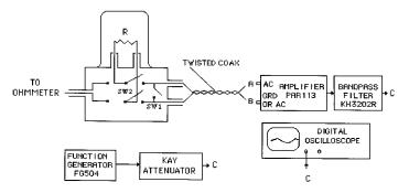
FIG. 5. Experimental apparatus.
