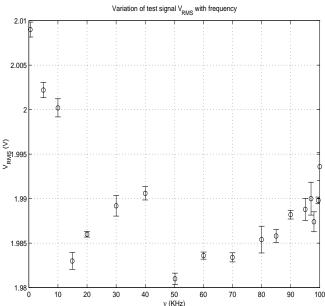
FIG. 6. RMS voltage  $V_{\rm RMS}$  produced by function generator as a function of frequency.
