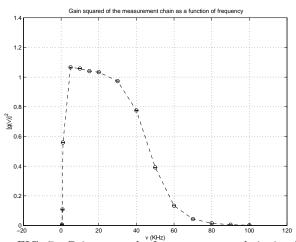
FIG. 7. Gain squared of measurement chain in the frequency range (0.5 KHz – 100 kHz.) **NOTE:** The dotted line is not a fitted function. Its purpose is tom emphasize a trend in the gain squared. The gain squared has been normalized such that the value of  $[g(\nu)]^2 = 1$  corresponds to a gain of 1000.
