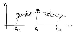
Fig. 1. Schematic of our model of an ideal string: a lattice of point masses joined by massless, linearly elastic springs with spring constants k. As a wave passes, the point masses  $m_j$  move from their equilibrium positions  $(X_j, 0)$  to  $(x_j(t), y_j(t))$ . In its undisturbed state,  $|X_{j\pm 1}-X_j|=l>a$ , where a is the relaxed length of each spring, so that a string under tension is modelled.
