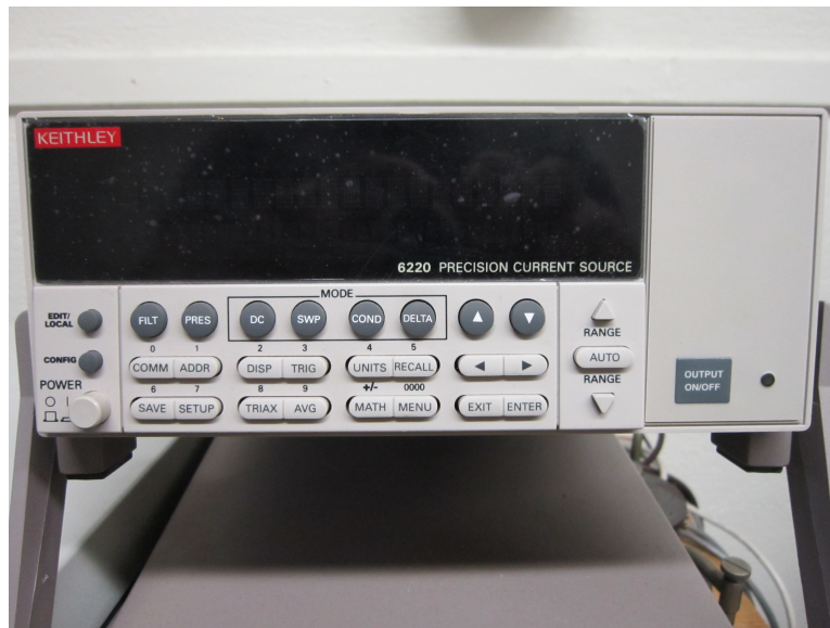
Figure 3: The control box for the 4-wire measurement.
